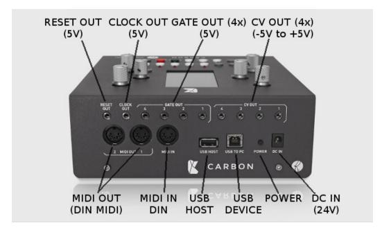
CARBON supports analog CV/gate, MIDI and USB MIDI connections so that you can make the most of your existing gear. All connections can be used at the same time. The function of the rear panel jacks and controls are as follows:
