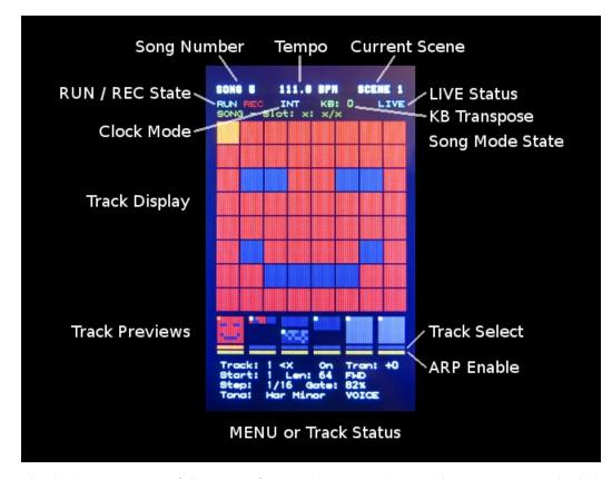
The display on CARBON follows a uniform and consistent layout. The screen area is divided into four sections:
